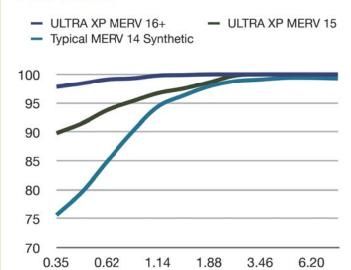
The efficiencies left show exceptional efficiency - the MERV 16+ Bag shows near HEPA performance with minimal efficiencies in the 0.3 micron range of 97.8%.
