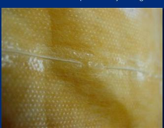
fiberglass media is backed by a thin layer of scrim to offer protection and durability.
